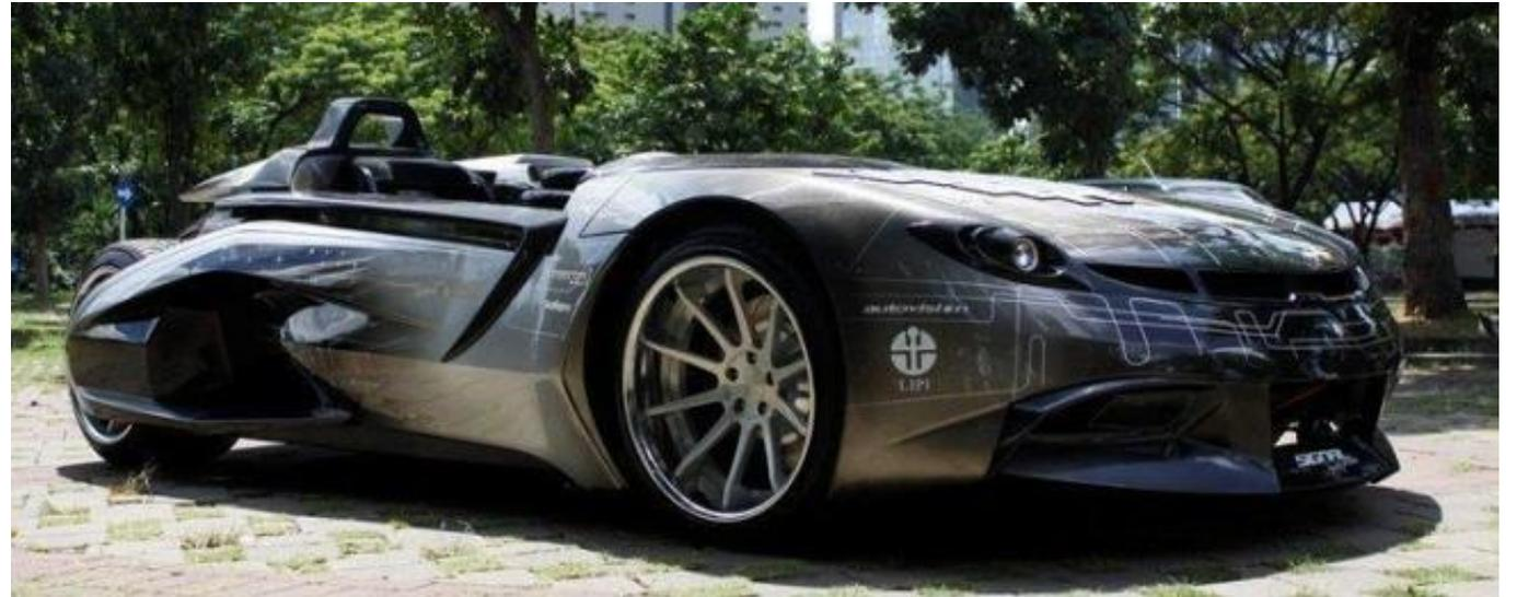
The SKEV-1 using 60 HP electric motor and having maximum speed of 140 km/h. Next generation of this supercar had been develop by Signal Custom Company is SV-1 as can be seen on the right picture.
