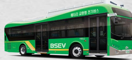
e-FIBIRD BSEV EV Low-floor Bus / Battery-Swapping
