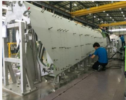
✈ B777 Fixed Leading Edge Inboard
